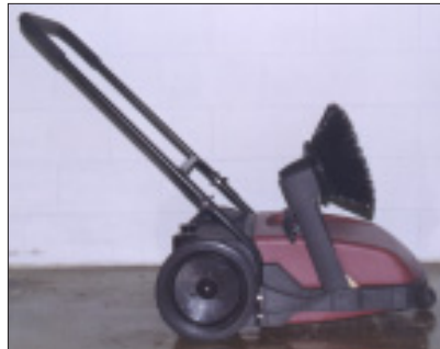
Side broom can be raised or lowered
